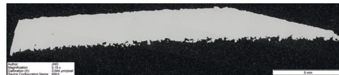
Figure 11: Crosscut high energy downskin exposure
