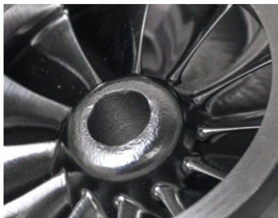
Figure 16: Top view of impeller after AFM
