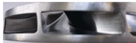
Figure 17: Detailed view of upskin surface after AFM
