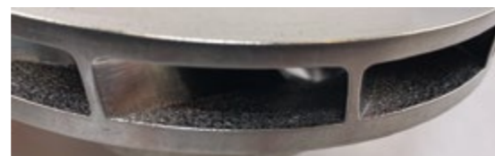
Figure 18: Detailed view of downskin surface after AFM
