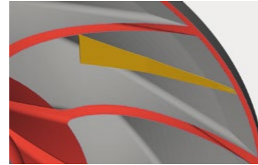
Figure 8: Bridging supports between blades
