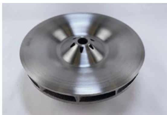
Figure 19: Bottom impeller surface after machining
